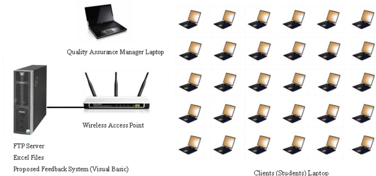
Fig. 1 the WLFS Infrastructure
